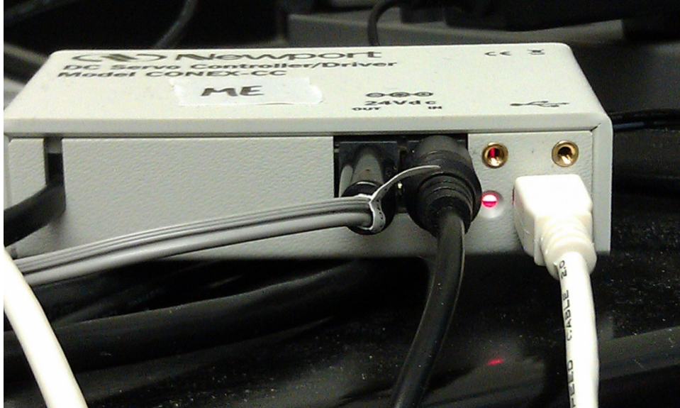
Figure: LED status is blinking red after executing 1PW1 command.
